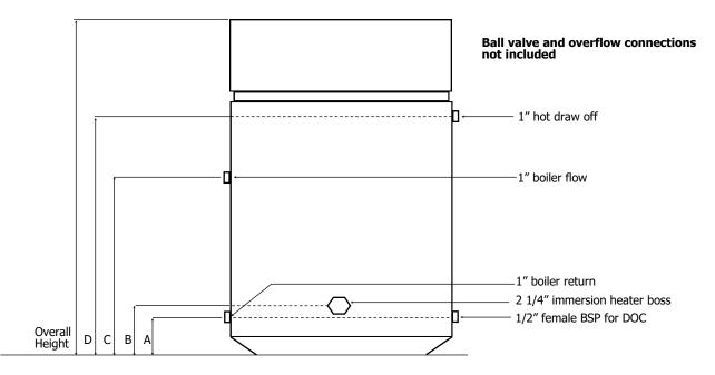
All dimensions are based on the cylinder shell only, insulation is not included
